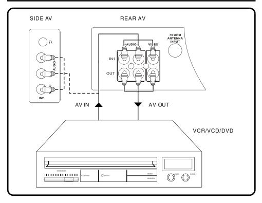
You can view the playback of VCR/VCD/DVD tapes by using the AUDIO and VIDEO INPUT sockets on the side or rear of the TV.
